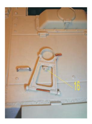
17. Install left air intake cover as shown
