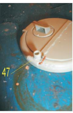
Install 1mm copper wire or paperclip handle as shown.
